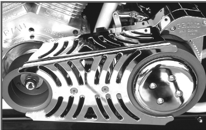
Tighten these bolts & torque to 29 foot pounds.
